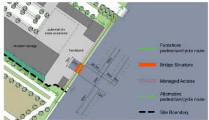
Figure 7.4. Wet well and berthing structure (Indicative/potential option)
